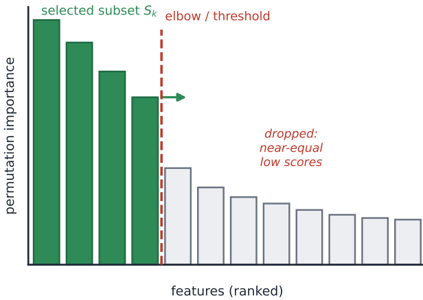
Figure 2. Random-forest importance ranks the candidate features and retains a compact top- k subset, forcing the downstream models to commit to the channels that carry signal rather than consuming every available feature.
